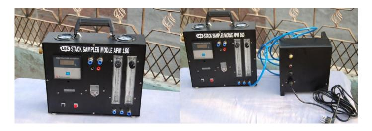
Monitoring of stacks and vents are requirement to ensure that emission of air pollutants are within the limit prescribed by regulatory authorities. By regular monitoring of emission one can establish that functioning and performance of installed control system are within the designed limits. Emission data also helps in improving performance of Air Pollution Control System energy saving and helps in optimizing process operation.
