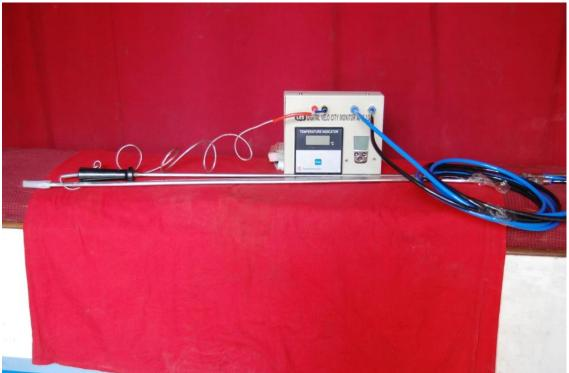
Digital Velocity Monitor Model APM-101 is designed to determine velocity of air/flue gas in duct /pipe/chimney. Where determination of the rate of flow inside a chimney is of interest. This instrument can be conveniently used to measure the total quantity/volume of emissions.
